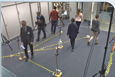
Lab testing at Fraunhofer FKIE to see how robust the security assistance system is: it must be able to clearly identify the carrier of a dirty bomb without sounding a false alarm.
