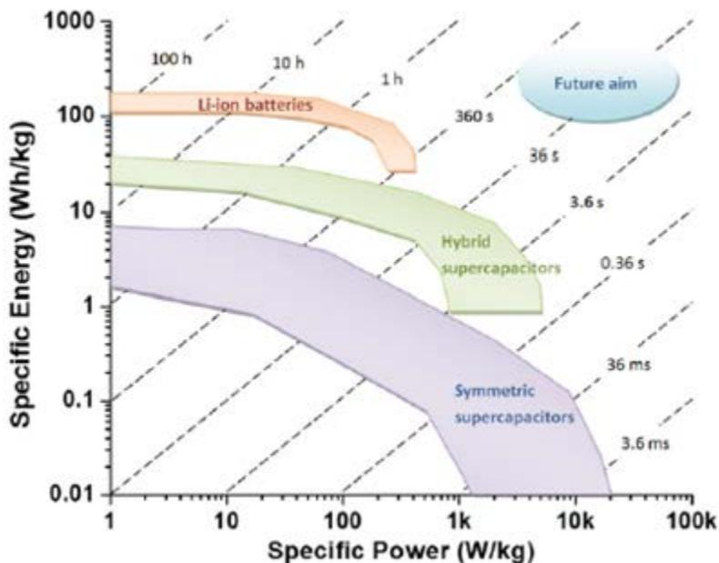
**Figure 1:** Ragone plot of energy density vs. power density for batteries and different types of today’s supercapacitors. These describe different varieties of supercapacitors and the future aim of the field: to achieve parity in energy density with high-performance batteries. Figure derived from (Tiruye, 2014)
